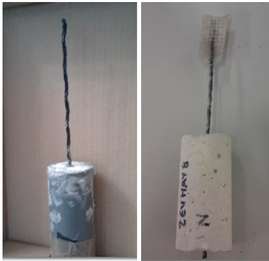
Fig. 5 - Production of specimens for tests pull out
