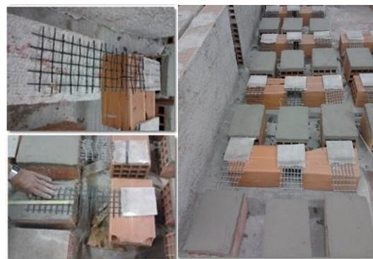
Fig. 10 – Application of meshes on masonry samples
