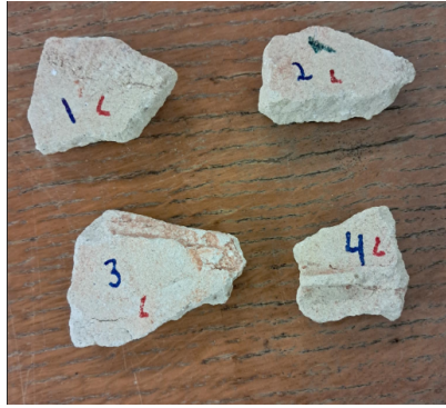
Fig. 3 | Samples for density and open porosity tests.
