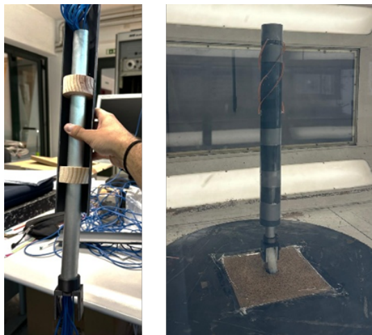
Fig. 1 | 0.2h-Gap model under testing – LNEC wind tunnel.
